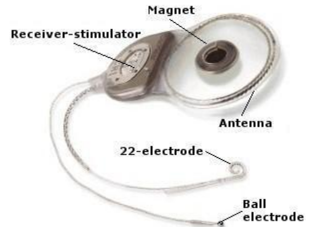
Figure 1. The internal component of the cochlear implant
